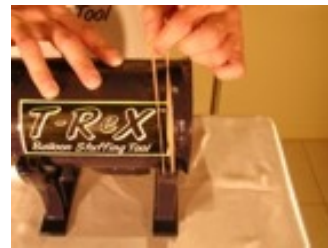
For extra strength - use elastic bands to secure body of T-Rex™ to Legs
