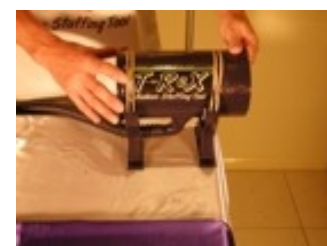
Place T-Rex™ in position if you are right handed put back of T-Rex™ to your right
